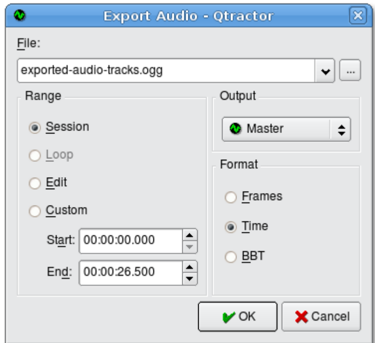
Illustration 3.16: Audio export window, where the audio tracks in a session can be named and exported as a single audio track in the particular format previously specified by the user in the View → Options window.
